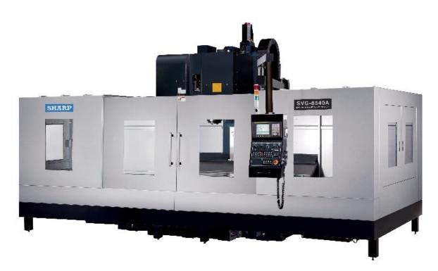
The Sharp SVG series was engineered from the ground up for hard metal machining. This is a extremely rigid "C" frame design using hardened and ground box ways. All structural components are made of Meehanite casting with internal ribs running throughout each section. Precision hand scraping of each section provides near perfect alignment assuring long term accuracies.
