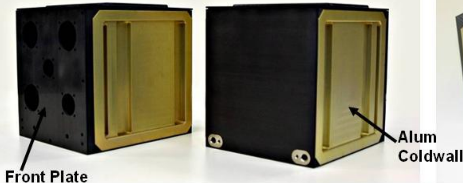
Assembled Composite Chassis with Aluminum Coldwall
