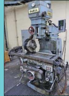
4 HP Doall Dovetail Ram Variable Speed Vertical Milling Machine
