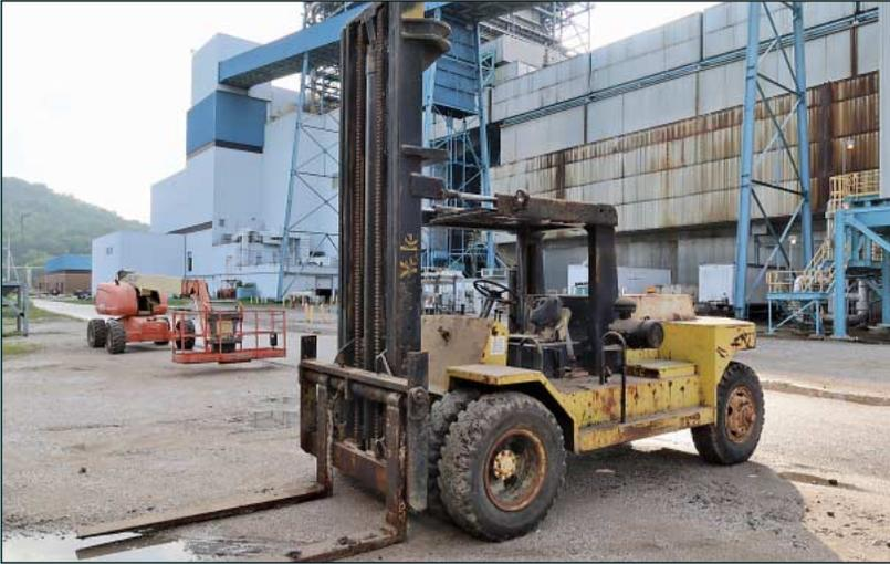
25,000 LB Yale Model GDP250E Diesel Pneumatic Tire Lift Truck
