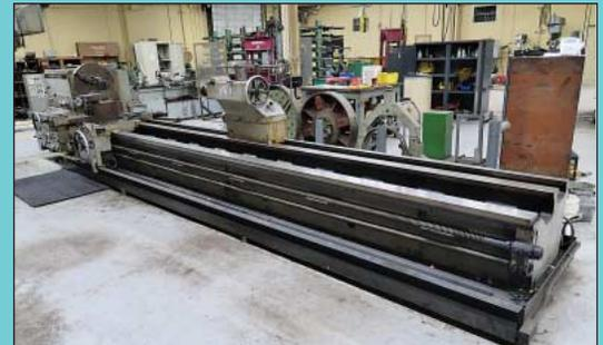
**40"/60" X 216" Clousing Model Trident 40" Geared Head Gap Bed Toolroom Engine Lathe**
