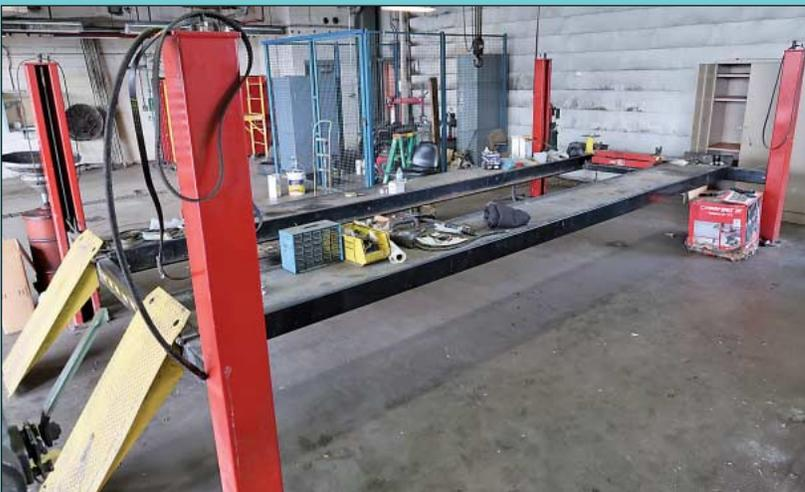
12,000 LB Ammco Model S412XSORI Drive on Type Vehicle Lift
