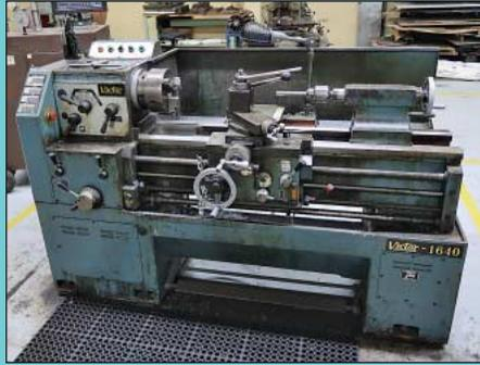
16" X 40" Victor Model 1640 Geared Head Toolroom Engine Lathe
