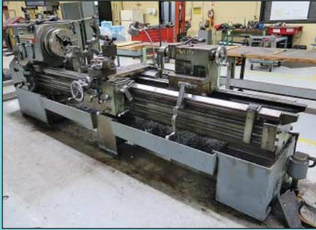
24" X 92" Leblond Regal Model 9" Hollow Spindle Geared Head Toolroom Engine Lathe
