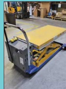
1,500 LB Vestil Portable Electric / Hydraulic Scissor Lift Table
