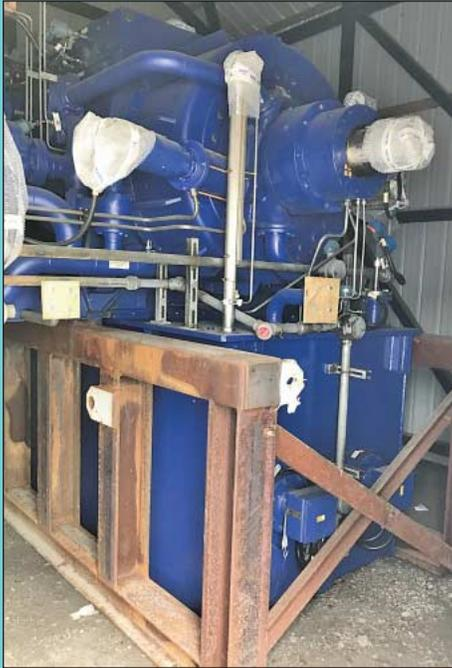
(2) Voith Type RW14-12C7 Variable Speed Planetary Gear
