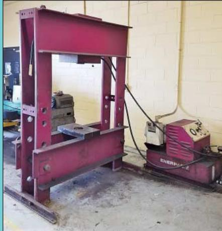
100 ton(est.) Enerpac Electric Hydraulic H-Frame Shop Press
