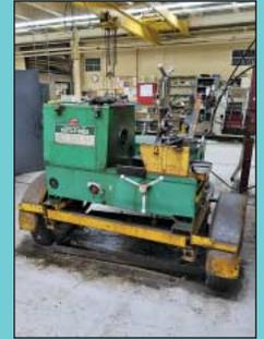
2" Oster Model 635 Pipe Mater Pipe Conduit and Bolt Threader
