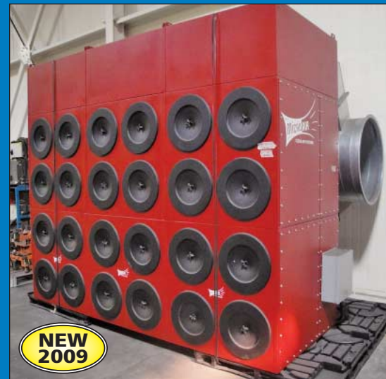
25 HP Micro Air Model RP8/3 24-Cartridge Dust Collector w/Pedestal
