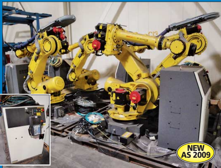
(7) Fanuc Model R 2000i Six-Axis Material Handling Robots ** (4) Brand New, Never Used **
