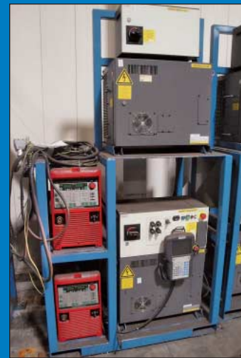
Close up of Fanuc R30i-A Master & Slave Controls w/ Fronius Trans Plus Synergic 4000 CMT Welders
