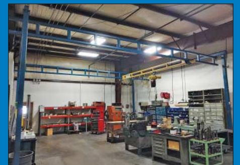
1,000 Lb. X 20' Span Gorbel Free Standing Overhead Bridge Crane System with 1/2 Ton Budget Electric Hoist, 30' Crane Runway with Uprights
