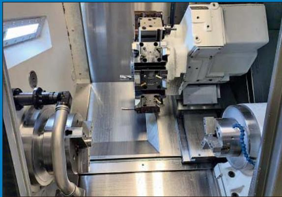
**Okuma Model LB3000EX II-MYW 450 Multi-Axis CNC Turning Center w/ Milling & Y-Axis;** s/n 209332, Okuma OPS-P300LA Control, 10" Chuck, 6" Sub Spindle, 12-Pos. Turret, 16.14" Max Turn Dia, 19.69" Max Turn Length, 5,000 RPM Spindle, Touch Setter, Parts Catcher, Chip Conveyor **(New 2017)**
