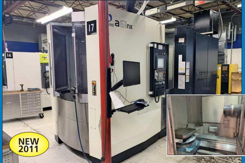
**Makino Model A61NX CNC Horizontal Machining Center w/ Full 4th Axis**
