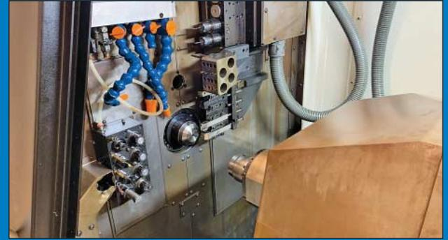
**(2) DMG Mori Model Sprint 32/8 Swiss CNC Turning Centers;** s/n 8107000192B and 8107000108B (2017), Fanuc 32i-Model B Control, Iemca Boss 338 HD Bar Feed, 2-Spindles, 2-Cross Slides, Y-Axis on Both Slides, C-Axis on Both Spindles, 32 mm Cap., 100 mm Main Spindle Z-Axis Stroke, 200 mm Counter Spindle Z-Axis Stroke, Counter Spindle Collet Cleaning, Sliding Headstock, Belt Type Chip Conveyor w/ Shaft Unloading Device, Mist Collector, Transformer (**New 2017 and 2018**)
