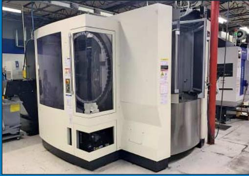
**Makino Model A61NX CNC Horizontal Machining Center w/ Full 4th Axis;** s/n 235, Professional 5-Control, 19.7" x 19.7" Dual Pallets, 28.7" X-Axis, 25.6" Y-Axis, 28.7" Z-Axis, 1,100 Lb. Pallet Cap., Full 360,000 Pos. 4th Axis, 60-Pos. ATC, 40 Taper, 14,000 RPM, Air Dryer, Broken Tool Sensor Outside Machining Area, Renishaw Probe, Upgraded Storage and Program Editing, Super GI Control, High Pressure Coolant, Chip Conveyor, Mist Collector (**New 2011**)
