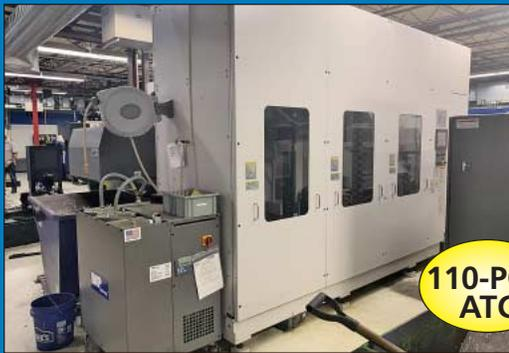
**Okuma Model MB-4000H CNC Horizontal Machining Center w/ Full 4th Axis;** s/n 155742, Okuma OSP-P200MA Control, 15.7" x 15.7" Dual Pallets, 22" X-Axis, 22" Y-Axis, 24.6" Z-Axis, 880 Lb. Pallet Cap., Full 360,000 Pos. 4th Axis, 110-Pos. ATC, 40 Taper, 15,000 RPM Spindle, Mayfran Concep 2000 Chip Conveyor, Tool Breakage Detection, Reinshaw Probe, Shower Coolant, TMAC Adaptive Control, Upgraded Storage and Program Editing, High Pressure Coolant, Chip Conveyor (**New 2011**)
