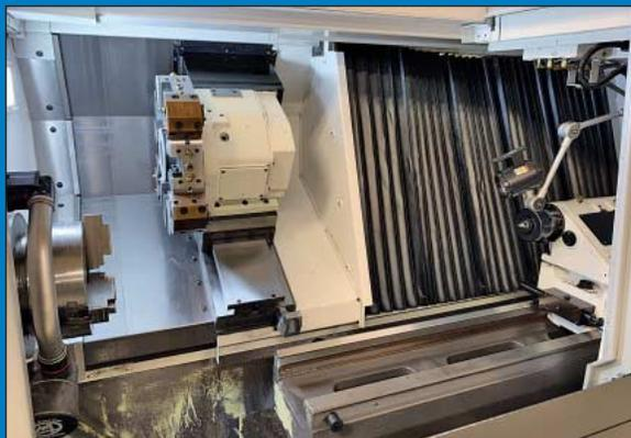
**Okuma Model Genos L3000-E Two-Axis CNC Turning Center;** s/n L3E0014, Okuma OSP-P300LAE Control, 10" Chuck, Tailstock, 13.39" Max Turn Dia., 43" Max Turn Length, 3,800 RPM Spindle, Upgraded MP Systems 1,000 PSI Coolant, Touch Setter, Mist Collector, Chip Conveyor **(New 2018)**
