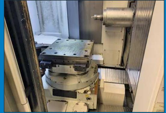
**Tongtai Model SH-4000P CNC Horizontal Machining Center w/ Full 4th Axis;** s/n TT040298, Fanuc Series Oi-MF Control, 15.7" x 15.7" Dual Pallets, 20" X-Axis, 20" Y-Axis, 20" Z-Axis, 880 Lb. Pallet Cap., Full 360,000 Pos. 4th Axis, 60-Pos. ATC, 40 Taper, 15,000 RPM Spindle, 400 PSI CTS, Micro-Broken Tool Detection in Magazine, Renishaw Probe, Upgraded Storage and Program Editing, High Speed Machining w/ Look Ahead, High Pressure Coolant, Chip Conveyor (**New 12 / 2017**)
