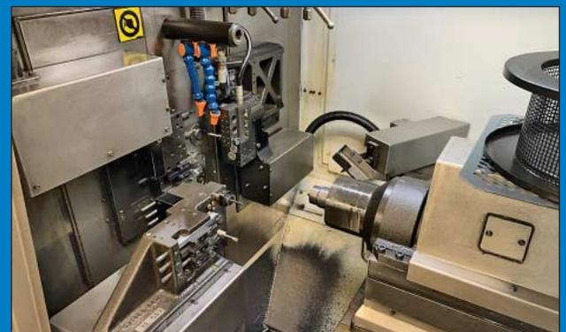
**DMG Gildemeister Model Speed 20-11 Linear 11-Axis Swiss CNC Turning Center;** s/n 8085012057B, Fanuc 160i Control, Iemca Ideal 325 Bar Feed, 240 mm Main Spindle Z-Axis Stroke, 300 mm Counter Spindle Z-Axis Stroke, 28.5 mm Counter Spindle Machining Dia., Counter Spindle Collet Cleaning, Kit for Bar Machining to 25 mm, Transformer, Mist Collector (**New 2011**)
