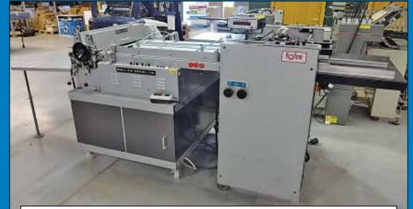
30" Rollem Model TR30 Die / Score System, Perforating /Scoring /Creasing /Slitting Machine
