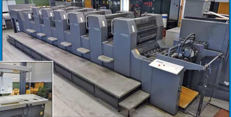
20" x 29" Heidelberg Model Speedmaster SM74-6-P3+L Six-Color Perfector Offset Printing Press w/Coating Tower
