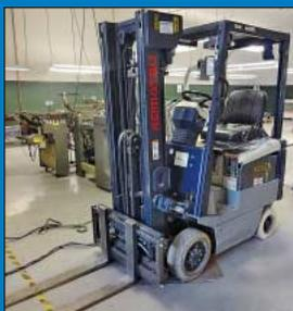
3,500 Lb. Komatsu Model FB18SH6 Electric Lift Truck
