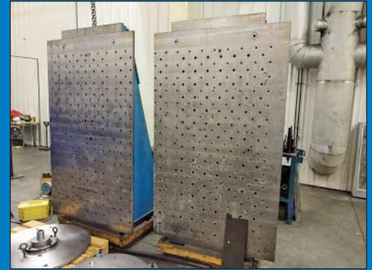
(2) 36" X 90" Angle Plates w/ 51" x 86" Drilled & Tapped Sub Plates
