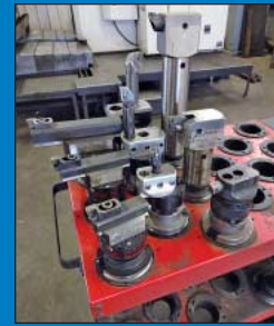
(3) D'Andrea TRM80 & TRM125 Adj. Boring Heads 50-Taper Toolholders
