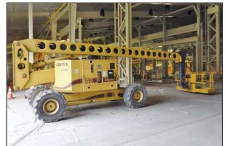
**80' Grove Model AMZ80XT Four-Wheel Drive Diesel Powered Hydraulic Manlift**
