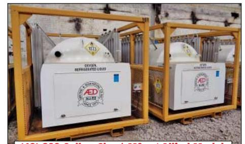
**(10) 800 Gallon Chart Mfg. / Allied Model HLD-900 Portable Liquid Oxygen Storage Tanks**
