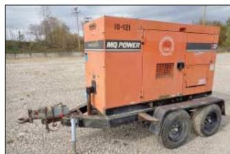
70 KW Multiquip Model DCA-70SSJU Whisperwatt Diesel Powered Trailer Mounted AC Generator
