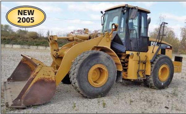
2005 Caterpillar Model 950G Articulating Rubber Tire Front End Loader
