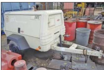
Ingersoll Rand Model XP185WJD Diesel Power Portable Air Compressor
