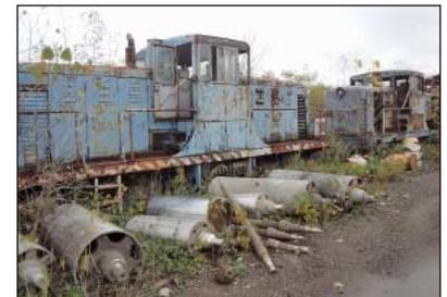
65 Ton and 44 Ton General Electric Diesel Locomotives
