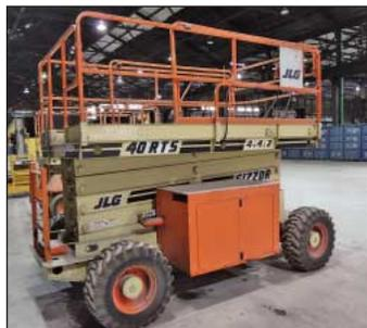
**40' JLG Model 40RTS 4X4X2 Four-Wheel Drive Diesel Powered All Terrain Scissor Lift**
