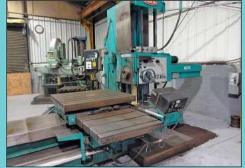
4" Shibaura Model BT10B-R1 Rotary Table Horizontal Boring Mill
