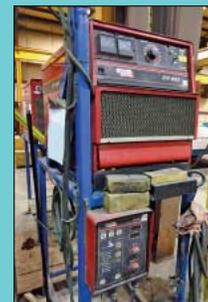
(15) Lincoln Model CV-655 Welders w/ LN-10 Wire Feeds
