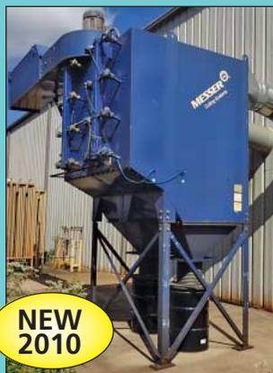
Messer Model DFT4-32 Cartridge Type Dust Collector
