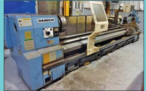
30" x 157" Dainichi Model DL-75X400 Flat Bed CNC Lathe
