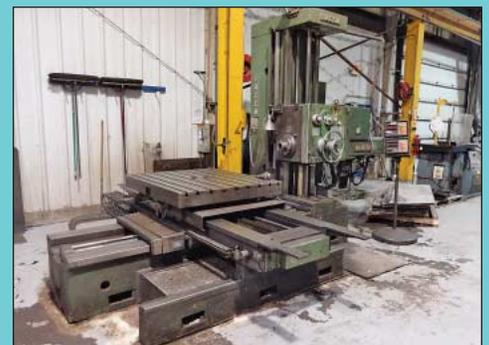
4" Sacem Hercules Model MST-XC-110 Rotary Table Horizontal Boring Mill
