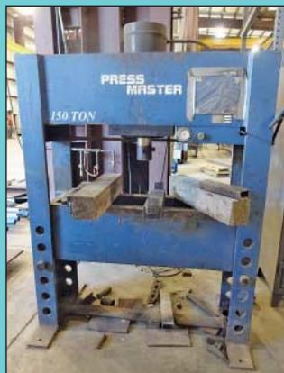
150 Ton H-Frame Press Master Hydraulic Press
