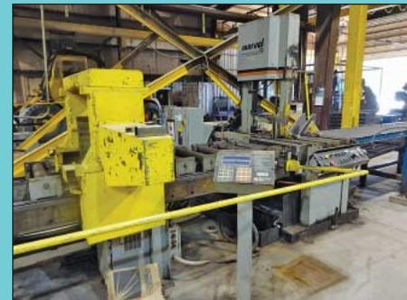
21" x 22" Marvel Model MV525PC/1 Automatic Tilt Frame Vertical Band Saw
