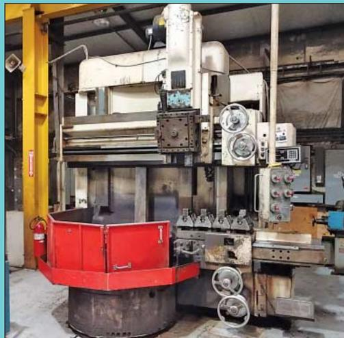
48" Bullard Model Cutmaster Vertical Turret Lathe
