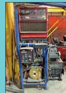
(2) Lincoln Model Powerwave 455 Welders w/ Wire Feed
