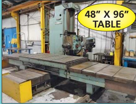
4" Nomura / Olympia Model B-100WB Four-Axis Table Type CNC Horizontal Boring Mill
