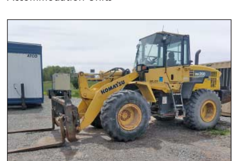
Komatsu Model WA250 to Articulating Rubber Tire 4-Wheel Drive Loader
