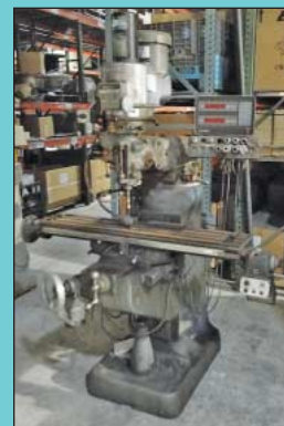
2 HP Bridgeport Variable Speed Vertical Mill
