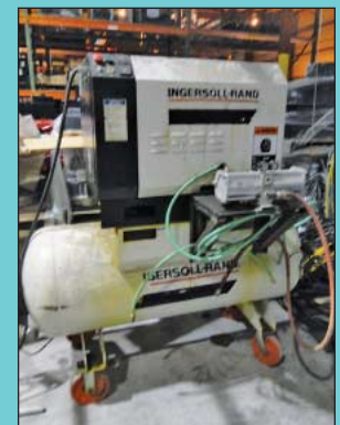
15 HP Ingersoll Rand Model SSR-EP15 Horizontal Tank Air Compressor
