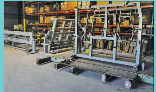
Approx. (25) Fire Truck (Green) and Condor Truck (Grey) Truck Cab Positioner Fixtures
