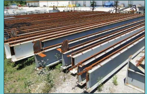
(60) Pieces of Assorted Size I-Beam Crane Rail Webs from 10" to 24", Flanges from 9" to 12"
