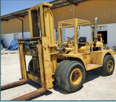
20,000 Lb. Power Lift Inc. Model ROF-20 Diesel Power Pneumatic Tire Lift Truck
