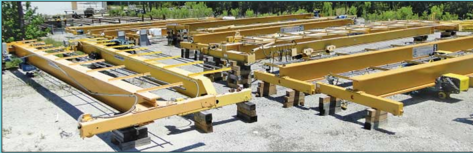
(15) 41' Span Eastern Crane Single Girder Top Running Bridge Cranes Up To 10 Ton
