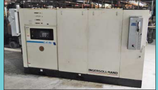
150 HP Ingersoll Rand Model SSR*XF150 Rotary Screw Cabinet Type Air Compressor
