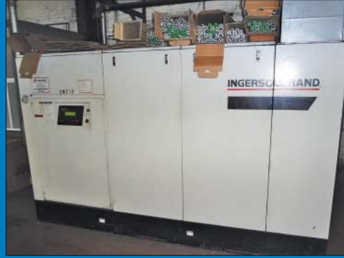
150 HP Ingersoll Rand Model SSR-EP150 Enclosed Rotary Screw Air Compressor
