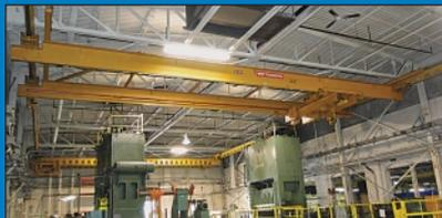
10 Ton X 50' Approx. Span Whiting Trambeam Double Girder Bottom Running Overhead Crane
