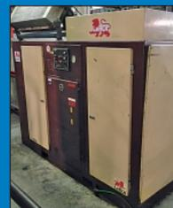
150 HP LeROI Model WE-1505S II Rotary Screw Cabinet Enclosed Type Air Compressor
