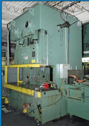
220 Ton Aida Model C2-20(2) Double Crank Gap Frame Press
