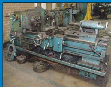
21-1/2" X 48" Cincinnati Tray-Top Geared Head Engine Lathe
