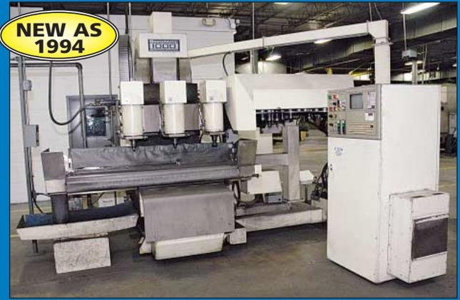
(2) Boston Digital Corp. Bostomatic 1000 Model 1741-3 Three-Spindle CNC Vertical Machining Centers
