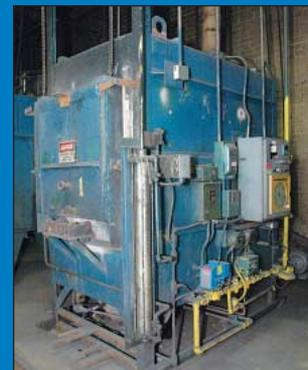
(4) Surface Combustion Electric Convection Tempering Furnaces
