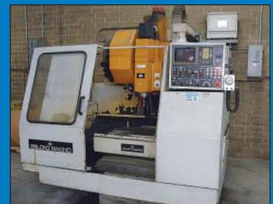
**Makino Model FNC60 CNC Vertical Machining Center**
