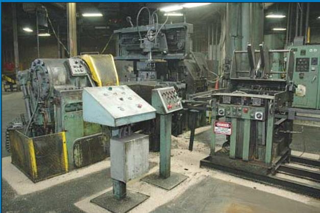
(5) 8,000 Ft. Lbs. Chambersburg Size 8MPC Impacter Horizontal Forging Machines
