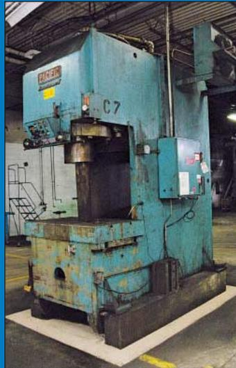
**375 Ton Pacific Model 375 PFII Pressformer Hydraulic Gap Frame Press**
