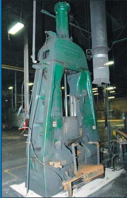
(2) 2,500 LB Chambersburg Ceco-Drop Model 25CD Forging Hammers
