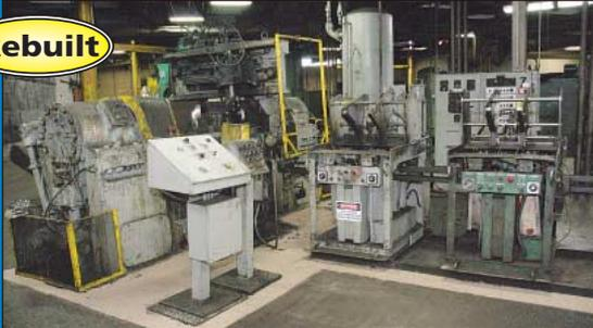
(5) 8,000 Ft. Lbs. Chambersburg Size 8MPC Impacter Horizontal Forging Machines
