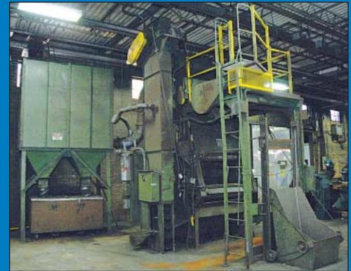
40" Dia. X 48" Wide Wheelabrator Tumblast Steel Belt Abrasive Blast Machine
