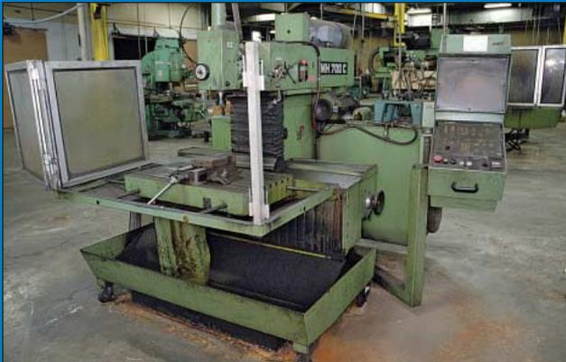
**Maho Model MH-700C CNC Horizontal Machining Center**
