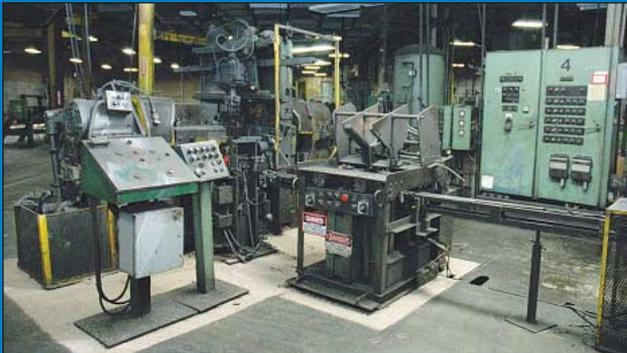
(2) 3,000 Ft. Lbs. Chambersburg Size 3MPC Impacter Horizontal Forging Machines
