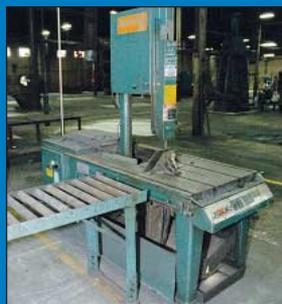
18" Marvel Series 8 Model MK1 Tilt Frame Vertical Band Saw
