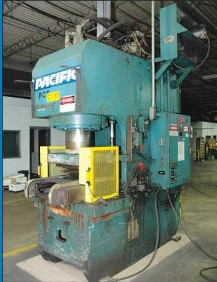
**(2) 250 Ton Pacific Model 250 PFII Pressformer Hydraulic Gap Frame Presses**
