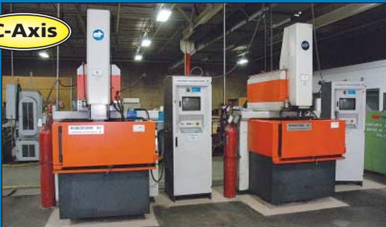
(2) Charmilles Model Roboform 40 Four-Axis CNC Die Sinker EDM's
