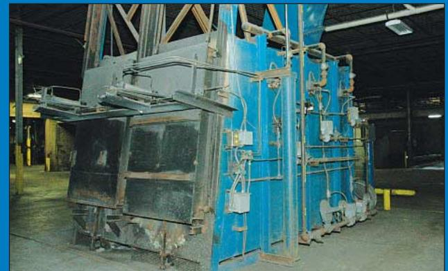
Air & Energy Systems Natural Gas Fired Dual Chamber Casting Pre-Heat Furnace
