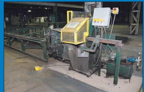
7/8" Bar Cap. X 12" Wide Blade Mfg. Unk. Hydraulic Alligator Style Shear
