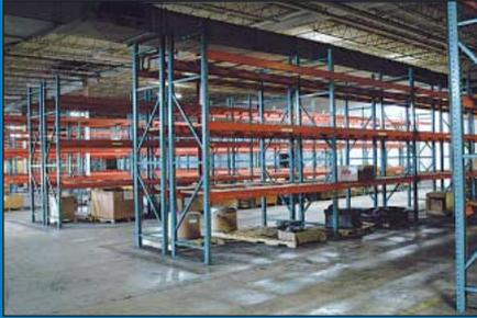
(91) Sections 120" W X 36" D X 144" H Adjustable Beam Pallet Rack
