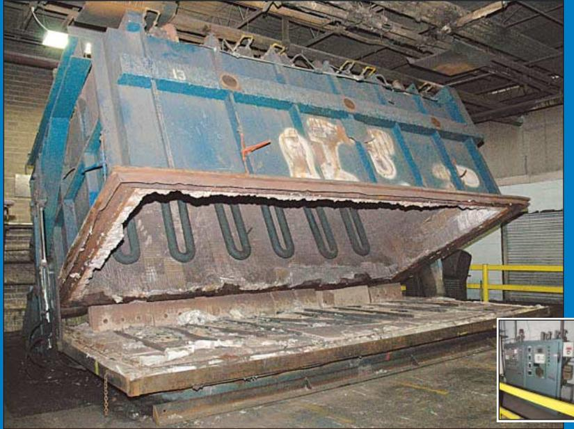
12' X 24' X 12'H Industrial Furnace Services Inc. Type Flip Up Natural Gas Fired Furnace
