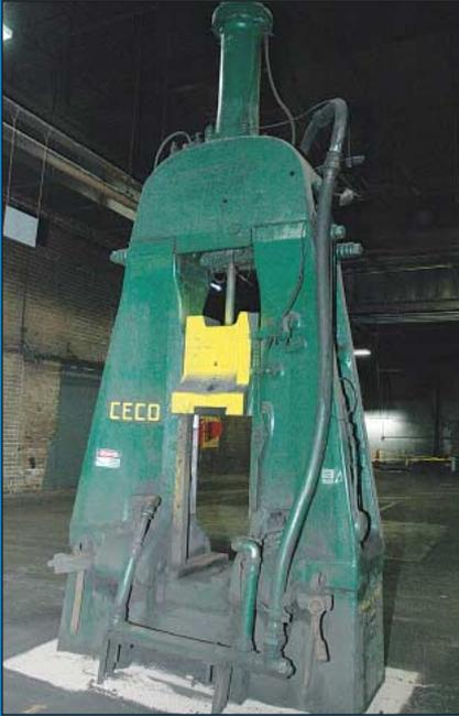
(4) 2,000 LB Chambersburg Ceco-Drop Model 20CD Forging Hammers
