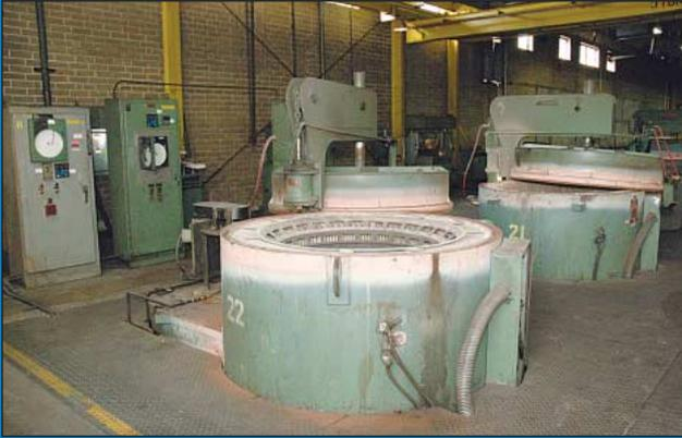
(4) 1,750 Degree Lindberg Model 12-R0-3836-174 Electric Fired Pit Type Furnaces
