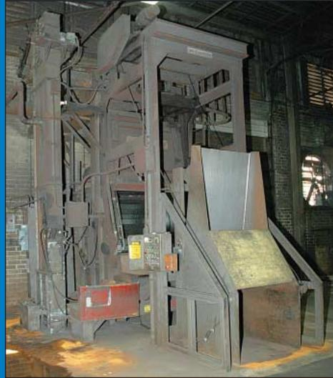
36" Dia. X 48" Wide Wheelabrator Tumblast Steel Belt Abrasive Blast Machine
