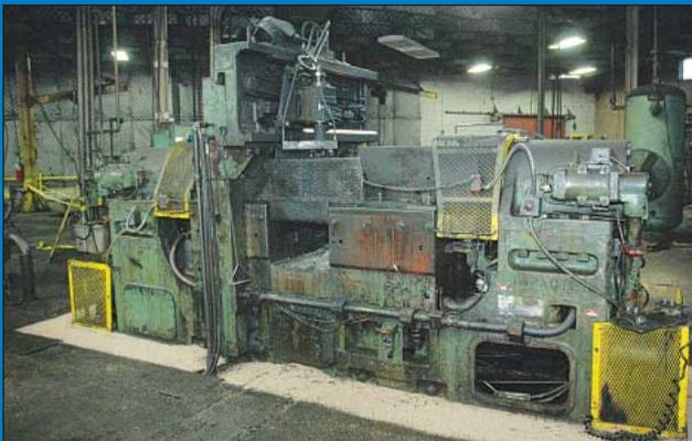
Reverse View (5) 8,000 Ft. Lbs. Chambersburg Size 8MPC Impacter Horizontal Forging Machines
