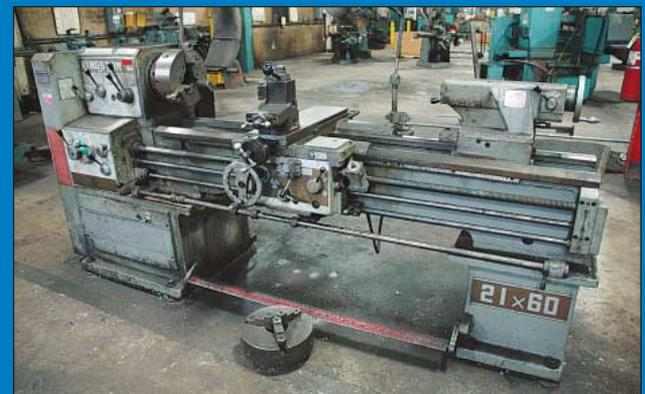
21" X 60" Kingston Model 2160 Geared Head Engine Lathe
