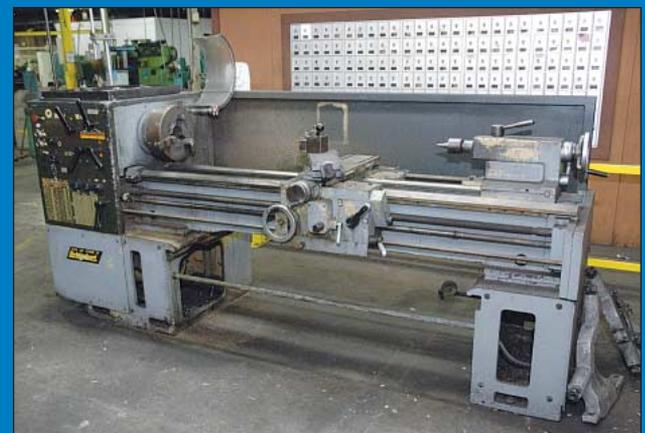
16" X 60" Bridgeport Romi Model 16-8 Geared Head Engine Lathe
