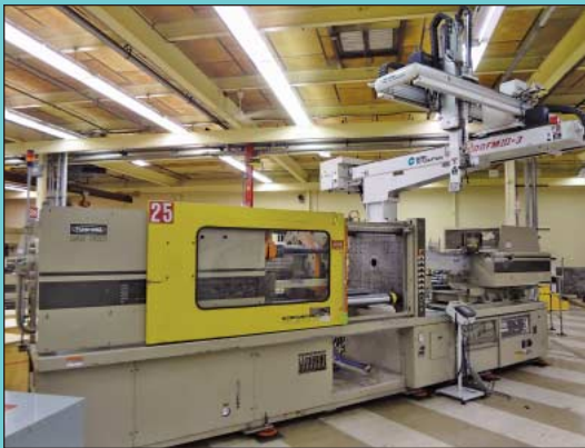
390 Ton x 41 Oz. Toshiba Model ISE390-17B Horizontal Hydraulic Clamp Plastic Injection Molding Machine
