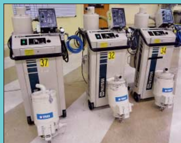
(5) Matsui Model JL4VC Jet Loader Vacuum Loading Systems
