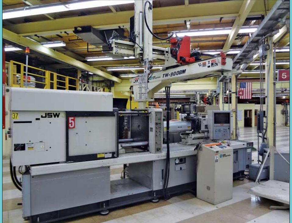
(2) 165 Ton x 11.8 Oz. JSW Model J165E-C5 Horizontal Toggle Clamp Plastic Injection Molding Machines
