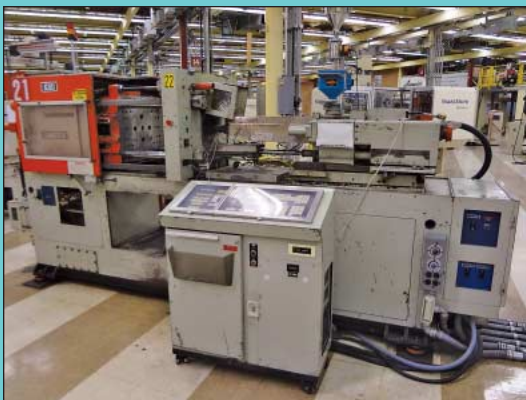
88 Ton x 4.5 Oz. Kawaguchi Model K-80-I Horizontal Toggle Clamp Plastic Injection Molding Machine
