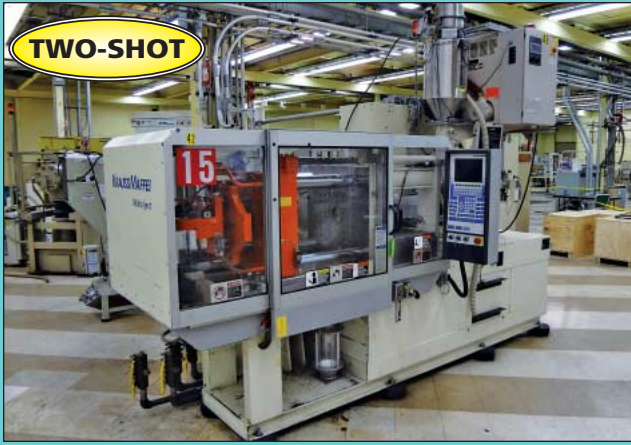
(2) 97 Ton x 1.66 Oz. x 1.66 Oz. Krauss Maffei Multijec Model KM80-160-90CL Hydraulic Two-Shot Plastic Injection Molding Machines
