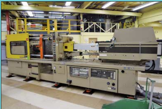
310 Ton x 41 Oz. Toshiba Model ISE310-17B Horizontal Hydraulic Clamp Plastic Injection Molding Machine
