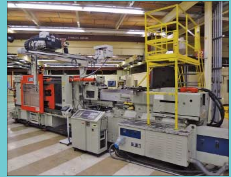
530 Ton x 66.9 Oz. Kawaguchi Model K-480-1 Horizontal Toggle Clamp Plastic Injection Molding Machine
