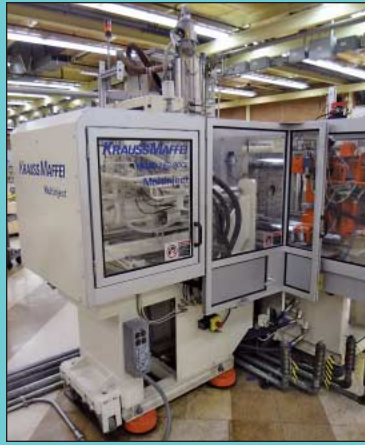
(2) 97 Ton x 1.66 Oz. x 1.66 Oz. Krauss Maffei Multijec Model KM80-160-90CL Hydraulic Two-Shot Plastic Injection Molding Machines
