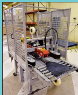
3M-Matic Model 800R Random Case Sealer Inline Box Taper
