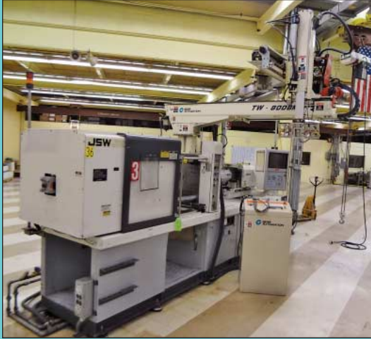
110 Ton x 5.6 Oz. JSW Model J110E-C5 Horizontal Toggle Clamp Plastic Injection Molding Machine
