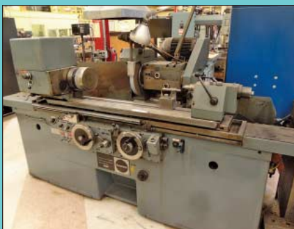
12" x 36" Karsten Series A Cylindrical OD Grinder
