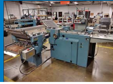
MBO B26 & B20 Continuous & Pile Feed Folders (1) w/ HHS Promelt Glue System, Horizon AFC-544AKT Cross Folder
