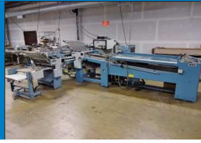
MBO B26 & B20 Continuous & Pile Feed Folders (1) w/ HHS Promelt Glue System, Horizon AFC-544AKT Cross Folder
