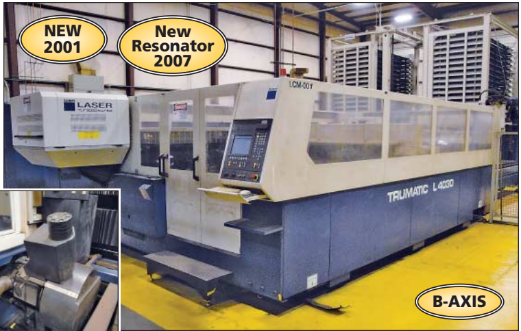
3,200 Watt Trumf Trumatic L4030 CNC Laser Cutting Machine w/ B-Axis
