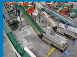
(7) 6" X 108" TEC HI626 Horizontal to Inclined Cleated Belt Conveyors
