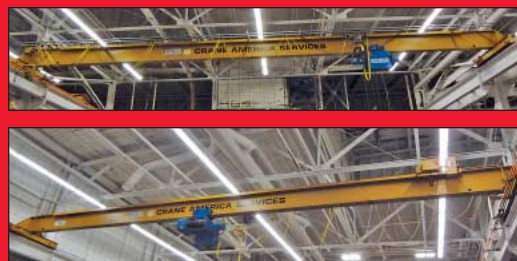
(3) 5 Ton X 48' Approx. Span Crane America Services Single Girder Top Running Overhead Bridge Cranes
