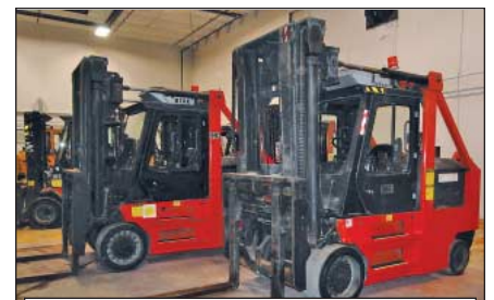
(6) 30,000 LB Taylor Model TCO-300S Big Red Cushion Tire Lift Trucks (New as 2008)
