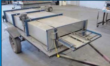
ESE Model Panelformer 100 Trailer Mounted Standing Seam Roof Panel Former
