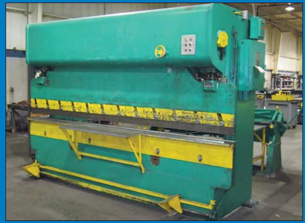
60 Ton X 12' Niagara Model IB-60-10-12 Mechanical Press Brake
