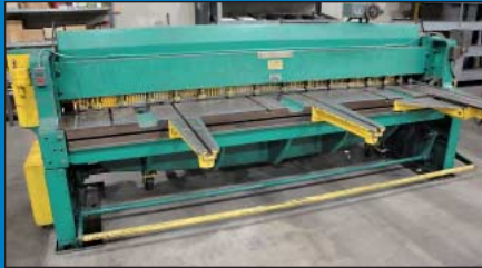
10' x 10 Ga. Wysong Model 1010 Mechanical Squaring Shear
