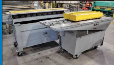
20 Ga. Engel Model 825 8-Stand Drives Flat-S Hammerlock and 20 Ga. Lockformer 10-Stand S-Lock Standing Seam
