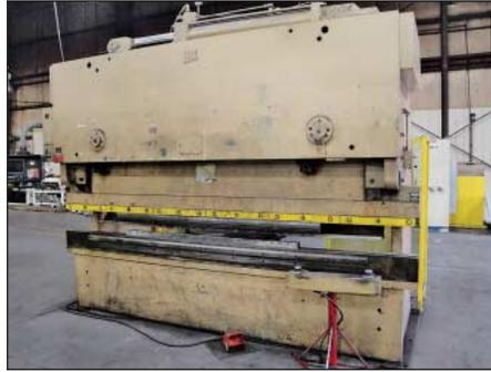
150 Ton X 12' HTC Model 150G Hydraulic Power Press Brake
