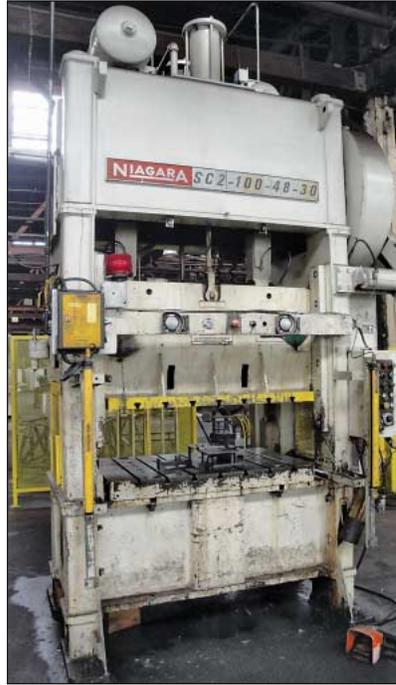
(2) 100 Ton Niagara Model SC2-100-48-30 Straight Side Double Crank Presses
