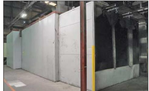
14' X 32' Approx. JR Greene Three-Pass Natural Gas Fired Combination Dry-Off and Cure Oven
