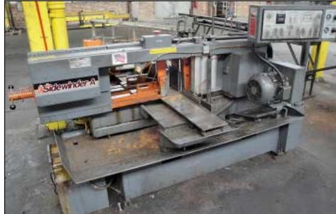
12" X 16" HEM Model Sidewinder Auto-4 Mitre Head Automatic Horizontal Band Saw
