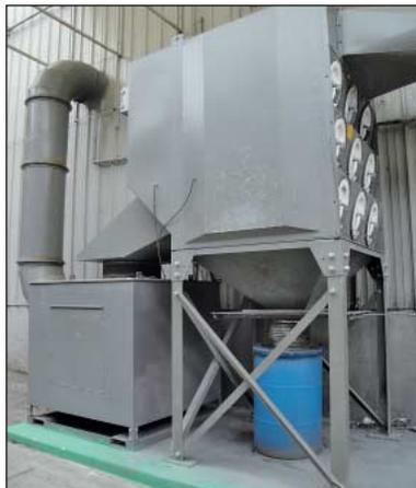
Gema 9-Cartridge Dust Collector w/ 5' X 5' X 5' Filter Box and 32" X 32" X 12' Long Indoor Filtration Unit
