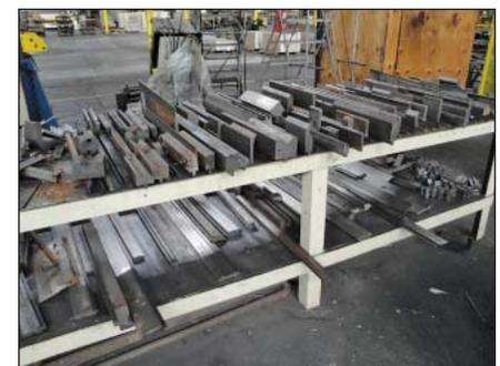
Partial View Large Quantity Press Brake Tooling
