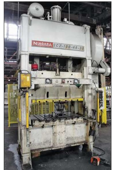
(2) 100 Ton Niagara Model SC2-100-48-30 Straight Side Double Crank Presses
