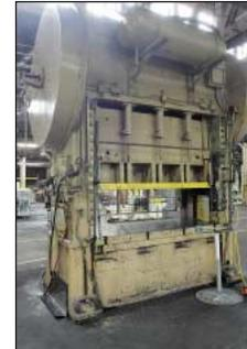
200 Ton Minster Model 50-7-84 Straight Side Double Crank Press
