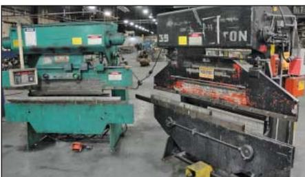
(3) 14 Ga. X 6' Diacro Hydra-Power Model 14-72 Mechanical Power Press Brakes
