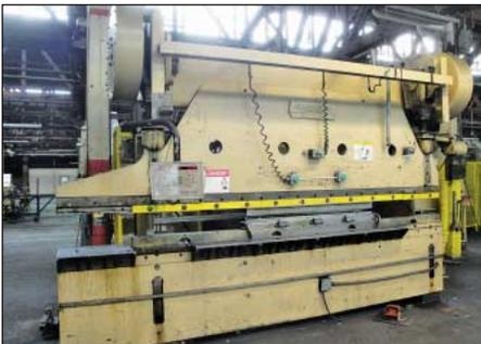
130 / 225 Approx. Ton X 14' Cincinnati Series 130X10 Mechanical Power Press Brake
