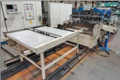
Schlatter Model MG12.4/4C Wire Mesh Welder
