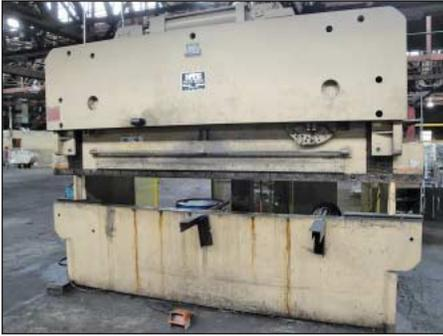
155 Ton X 12' HTC Model 155-12H Hydraulic Power Press Brake
