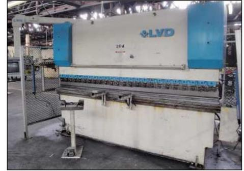
150 Ton X 124" LVD Type 150BH-10-MNC-95 Multi-Axis CNC Press Brake
