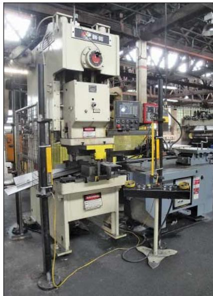
80 Ton Niagara Model Bison BN-80-OBS Variable Speed Gap Frame Press
