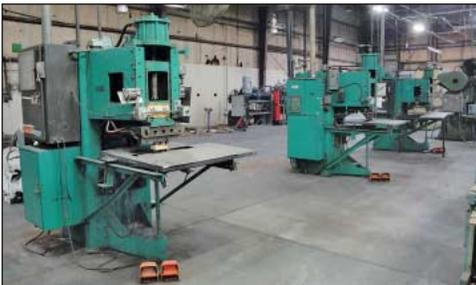
(3) 300 KVA Federal Type P3-24A Press Type Spot Welders
