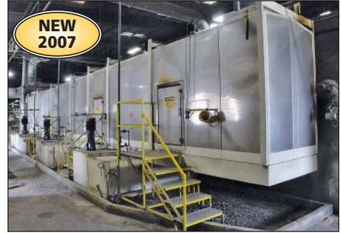
Col-Met Three-Stage Stainless Steel Pass-Thru Tunnel Type Parts Washer
