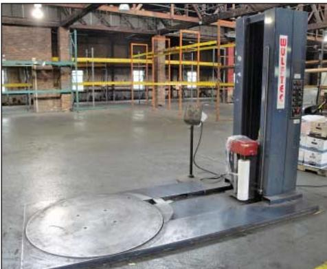
Wulftec Rotary Pallet Stretch Wrapper
