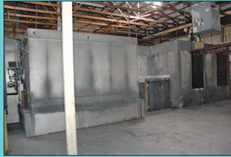
250' Mfg. Unk. Long Pass Thru Modular Panel Dry-Off Oven
