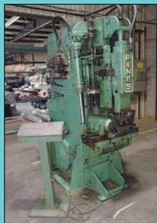
20 Ton Pines Model 20T Hydraulic Vertical Tube Bender
