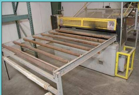
60" HMT Two-Roll Hot Roller Laminator
