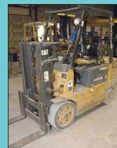
4,000 Lb Caterpillar Model GC20 Solid Tire LP Gas Lift Truck
