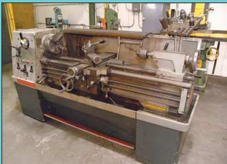
15" X 30" Clausing Colchester 15 Geared Head Engine Lathe
