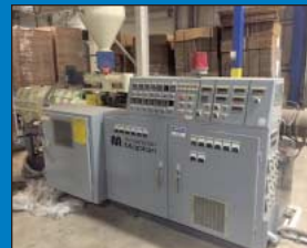
(2) 88 mm American Maplan Model TS88 Twin-Screw Extruders
