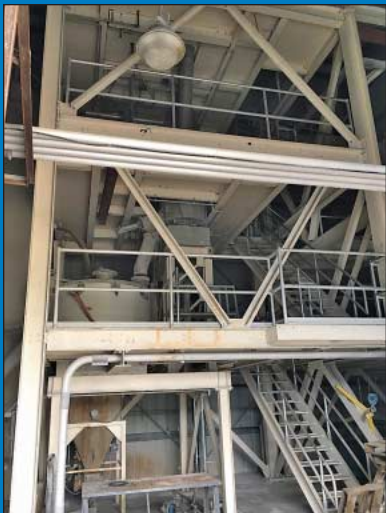
Henschel Model KM-1750 / FM-500 High Intensity Mixing System, 150-HP (Mfr. 1998 - Updated)
