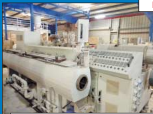
2" to 6" PVC Pipe Line w/ Techwell 114-MM Extruder (2007), Tanks, Puller, Saw, Beller and Bundler
