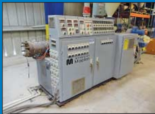
(2) 1/2" to 2" PVC Pipe Lines w/ American Maplan TS88 Extruders (1998), Tanks, Puller, Saw, Beller and Bundler
