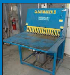
36" Profab Model Cleatmaker II Hydraulic Cleat Bender
