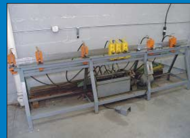
10' X 16 Gauge Lockformer Model Speed Notch Eight-Head Notching System
