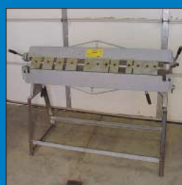
48" Central Machinery Finger Brake
