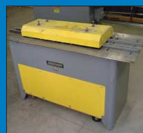
9-Stand Lockformer Model Cleat Former Double End Roll Forming Machine
