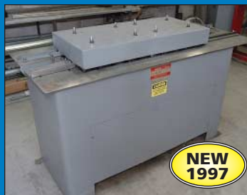
10-Stand Flagler Model 22 GA-QF Quad Form Roll Forming Machine
