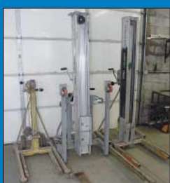
(2) Genie Superlift Model SLC-18 Aluminum Frame Cable Type Material Lifts
