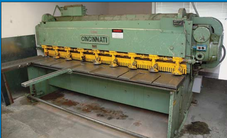
8' X 10 Gauge Cincinnati Model 1008 Hydraulic Squaring Shear
