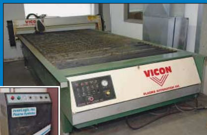
60" W X 120" Long Plasma Automation Vicon Dual Twin Drive Plasma Cutting Table
