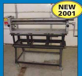
50" X 16 Gauge Enco Model 130-5501 Manual Slip Roll
