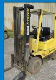
3,000 LB Hyster Model H30XM LP Gas Pneumatic Tire Lift Truck
