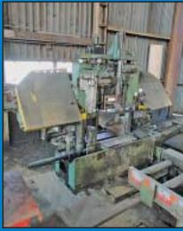
16" X 20" Behringer Model HPB420 Mitre Base Double Column Horizontal Band Saw
