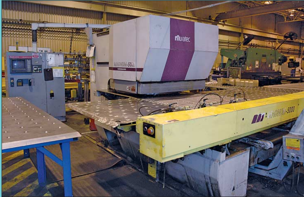
55 Ton Murata Wiedemann Model M-5000P460052 CNC Turret Punch
