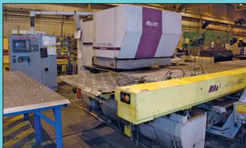
55 Ton Murata Wiedemann Model M-5000P460052 CNC Turret Punch
