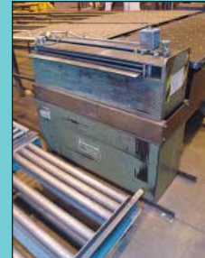
40" Wide Gauer Model 5H-40 Sheet Edging Machine
