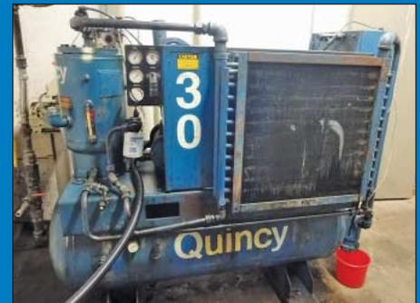
30 HP Quincy Model 30 Rotary Screw Horizontal Tank Air Compressor
