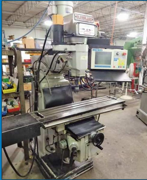
3 HP Cleveland Three-Axis CNC Vertical Milling Machine
