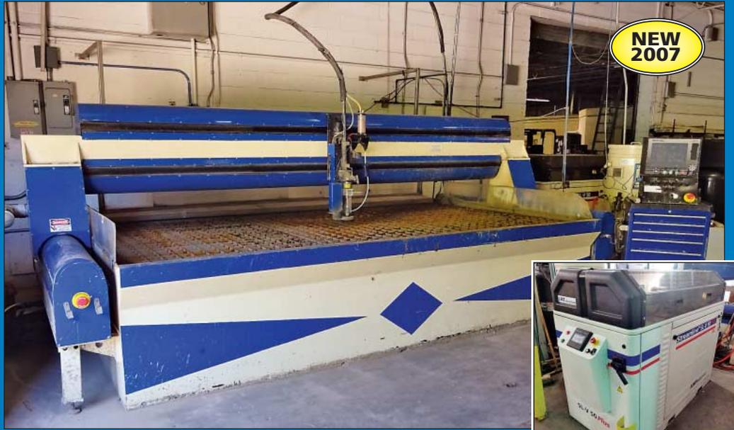
6' x 13' Ward Jet Model Z613 CNC Water Jet Cutting Machine
