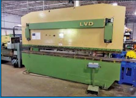
150 Ton x 13' LVD Model 150JS13 Hydraulic Power Press Brake w/ CNC Back Gage
