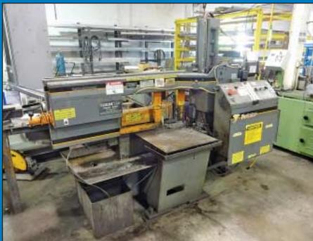
14" x 20" HEM Model Twister Miter Head Horizontal Band Saw
