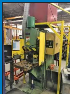
100 KVA NSRW Vertical Press Type Spot Welder
