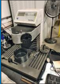
Trumpf Quickset ZS01 Tool Presetter
