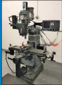
3 HP Alliant Model RT2 CNC Vertical Milling Machine
