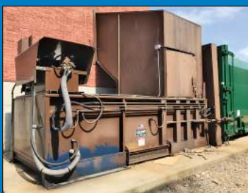
Marathon RJ450HDC Horizontal Hydraulic Trash Compactor
