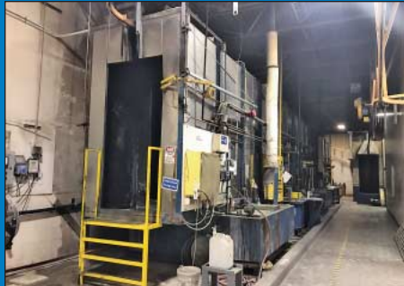
42" x 92" Window x 75' Long Ramco Finishing System Nine-Stage Pass-Thru Tunnel Washer
