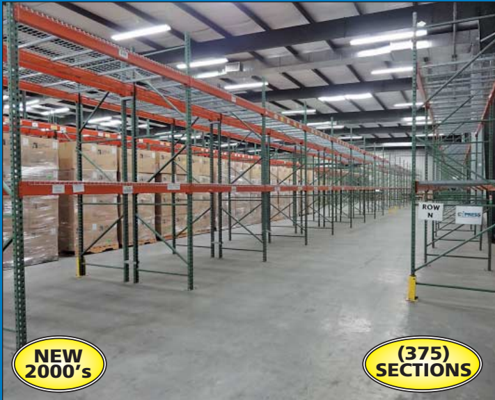
(375) Sections 42" Deep X 96" Wide X 144" High Wireway Husky Invincible Tear Drop Style Adjustable Beam Pallet Rack
