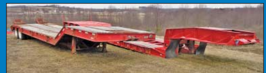
2001 / 35 Ton Talbert Model TLW-35-FG-1-T1 Lowboy Trailer
