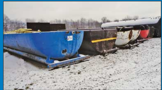
(6) 10' Wide X 40' Long Open Top Storage Vessels – Approx. 7,000 Gallons
