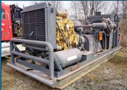
Joy Model WB-12 Piston Type Air Booster, Cat 3406 Engine, Unit 8053
