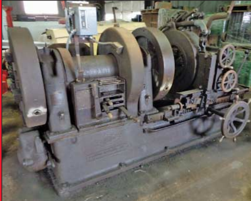
8-5/8" Landis Receding Chaser Semi-Automatic Pipe Threading and Cutting Machine
