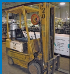
2,500 Lb TCM Model FCG15N5 LP Gas Solid Tire Lift Truck
