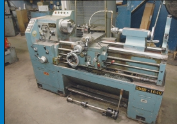
16" X 40" Victor Model 1640 Gap Bed Engine Lathe
