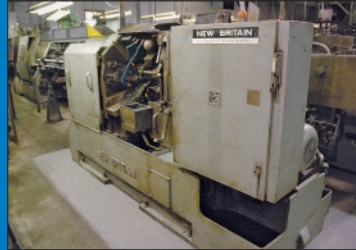
1" New Britain Model 51 Six Spindle Automatic Bar Machine
