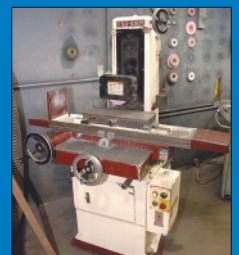
6" X 18" Chevalier Model FSG-618M Hand Feed Surface Grinder
