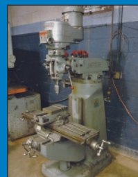
2 HP Bridgeport Series I Vertical Milling Machine
