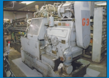
(2) 9/16" Acme Gridley Model RA-6 Six Spindle Automatic Bar Machines
