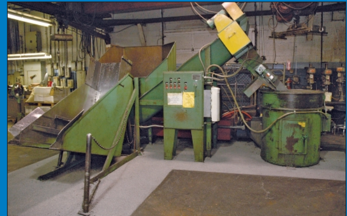
Reclament Oil Recovery System Chip Processing System
