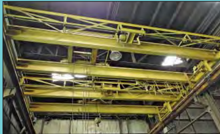
(3) 7 -1/2 Ton X 26' Approx. Span Pelham Double Girder Top Running Overhead Bridge Cranes; (2) w/Remote Controls
