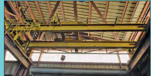
(3) 7 -1/2 Ton X 26' Approx. Span Pelham Double Girder Top Running Overhead Bridge Cranes; (2) w/Remote Controls
