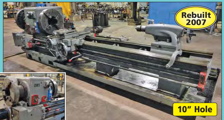
25" X 120" Dean Smith & Grace Model 25P Hollow Spindle Geared Head Engine Lathe
