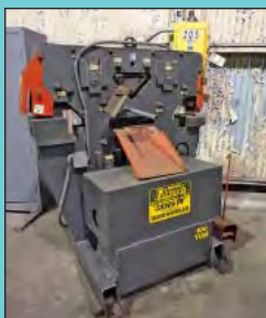
100 Ton Edwards Model Jaws IV Hydraulic Ironworker
