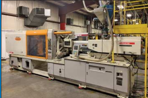
396 Ton X 44 Oz. Kawaguchi Model KM360B2 Toggle Clamp Plastic Injection Molding Machine
