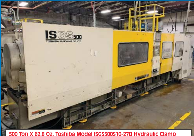
500 Ton X 62.8 Oz. Toshiba Model ISGS500S10-27B Hydraulic Clamp Plastic Injection Molding Machine
