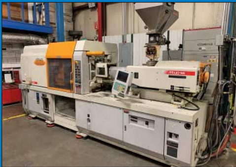
154 Ton X 9 Oz. Kawaguchi Model KM140B2 Toggle Clamp Plastic Injection Molding Machine
