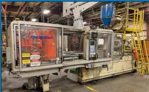
350 Ton X 34 Oz. Krauss Maffei Model KM350-1900C2 Hydraulic Clamp Plastic Injection Molding Machine
