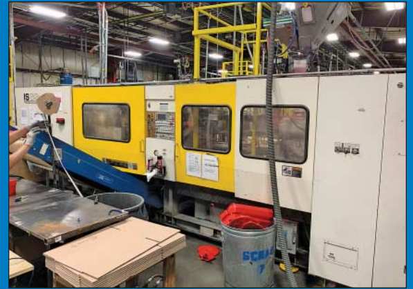
390 Ton X 30.2 Oz. Toshiba Model ISGS390-i19A7 Hydraulic Clamp Plastic Injection Molding Machine
