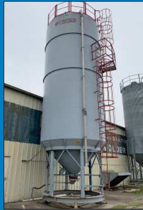
12' Diameter X 30' High Approx. Corrugated Steel Material Storage Silo Mounted on Weight Scale Base
