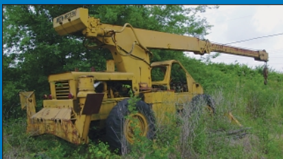
Austin Western Diesel Engine Rubber Tire Yard Crane
