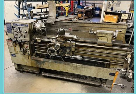
18" x 60" Sharpe Model 1860C Engine Lathe
