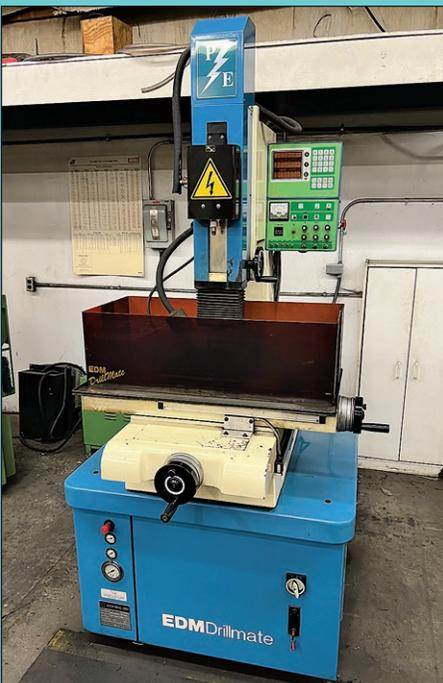
Seven Metal Corp EDM Drillmate 1376 EDM Hole Popper
