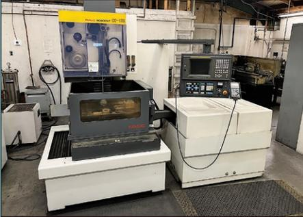
Fanuc Robocut Alpha-1B CNC Wire EDM
