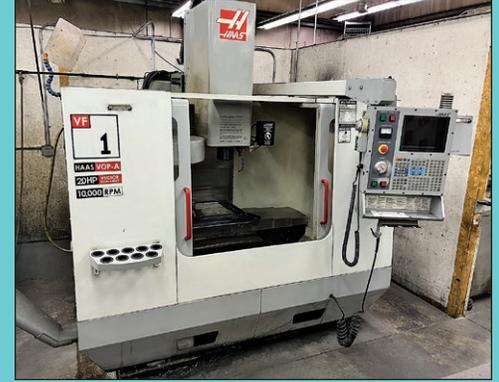
Haas Model VF-1D CNC Vertical Machining Center
