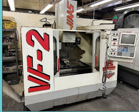
Haas Model VF-2 CNC Vertical Machining Center
