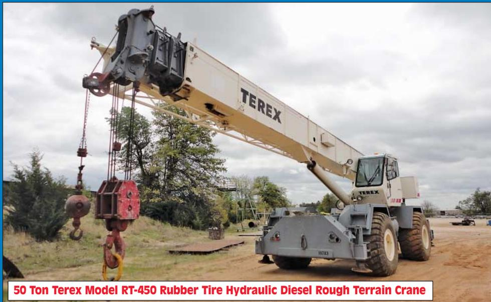
**50 Ton Terex Model RT-450 Rubber Tire Hydraulic Diesel Rough Terrain Crane**
