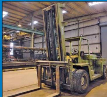
30,000 Lb. Clark Model Y2030 Pneumatic Tire Diesel Forklift
