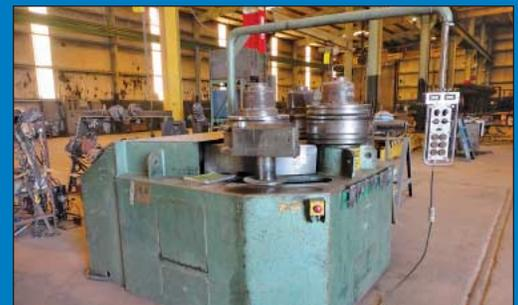
**6" X 6" X 5/8" Roundo Model R6S R-6-S Horizontal Hydraulic Angle Bending Roll**
