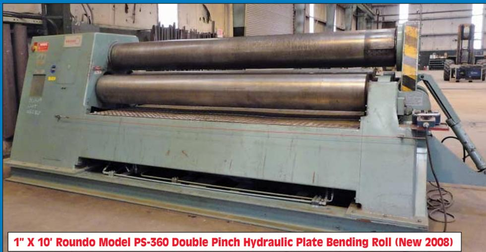
**1" X 10' Roundo Model PS-360 Double Pinch Hydraulic Plate Bending Roll (New 2008)**
