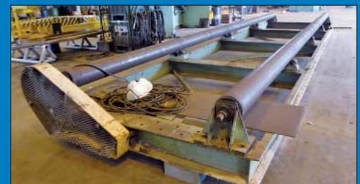
20,000 Lb. X 30' Mfg. Unk. Steel Roller Motorized Turning Roll
