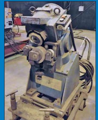
Gullco Model GBM-25 Portable Plate Beveling Machine
