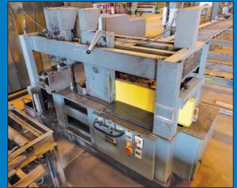
36" Trennjaeger Model PMC12-F Automatic Upacting Cold Saw
