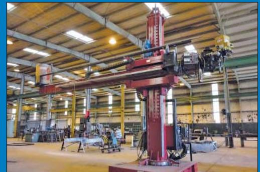
**13' X 13' Key Plant / Red-D-Arc Model THD-5MX5M Welding Manipulator (New 2012)**
