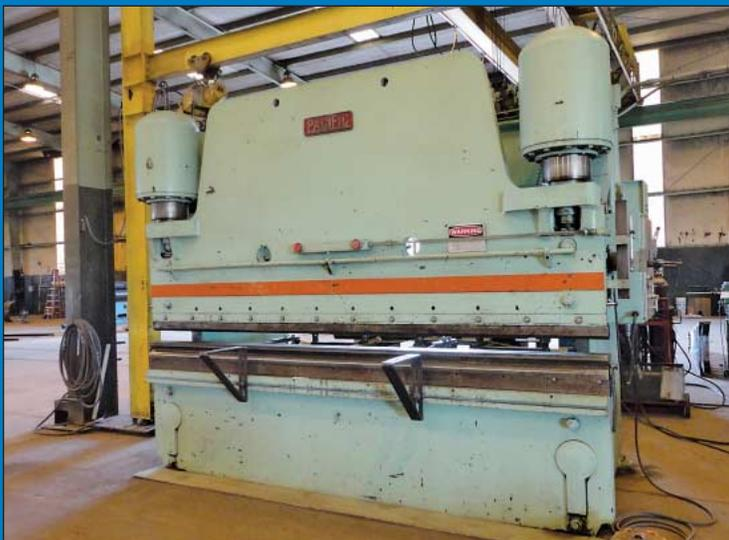
400 Ton X 12' Pacific Model K400-12 Hydraulic Power Press Brake
