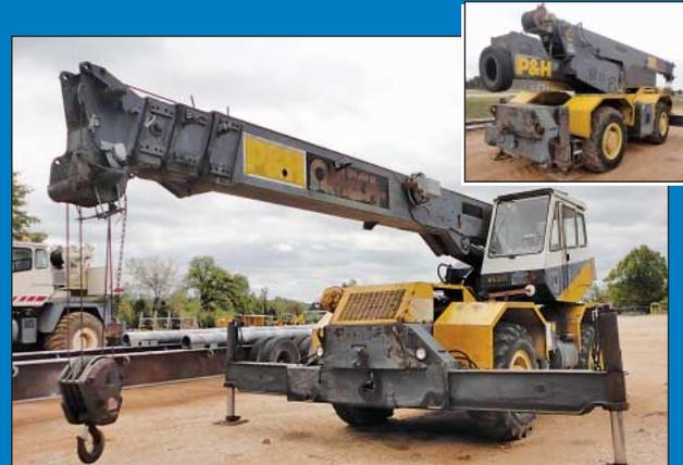
20 Ton P&H Omega 20 Model OM-20 Rubber Tire Hydraulic Diesel Rough Terrain Crane
