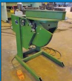
2,000 Lb. CWI Model P200F Tilting and Rotating Welding Positioner
