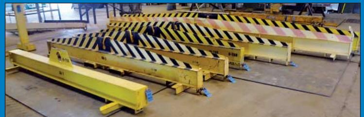
Large Quantity of Lifting Equipment including Magnetic Plate Handler, Spreader Bars and Related.
