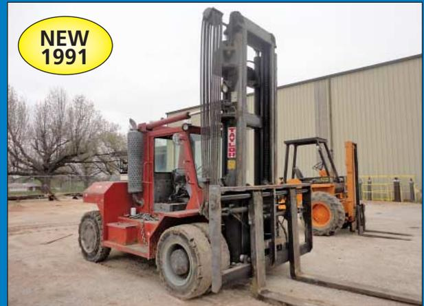
25,000 Lb. Taylor Model TE-250S Pneumatic Tire Diesel Forklift
