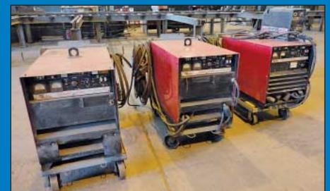
(9) Lincoln Electric Model Idealarc DC-600 Welding Power Sources
