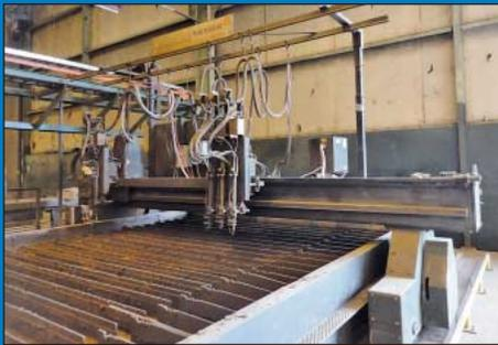
12' X 64' Messer Model TMC-4512 CNC Plasma Oxy Cutting Table
