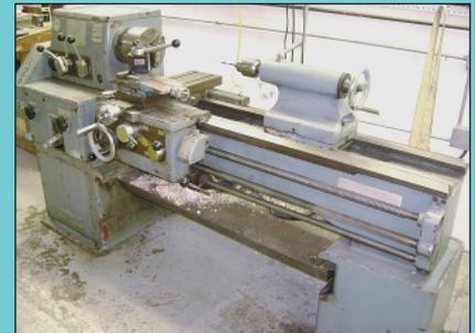
17" X 40" AFM Type Tue40 Engine Lathe
