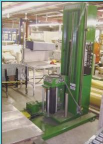
Highlight Model Synergy 3 Power Hydro Rotary Pallet Stretch Wrapper
