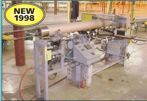
Rockport Machine Co. Model W1 Tube Winder
