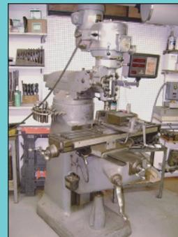
(2) 1-1/2 HP Bridgeport Variable Speed Milling Machines
