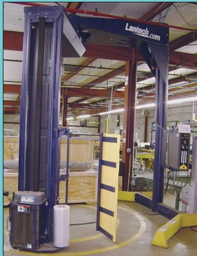
Lantech Model S-300 Rotary Arm Semi-Automatic Stretch Wrapper
