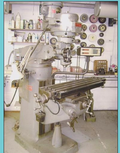
2 HP Bridgeport Variable Speed Milling Machine
