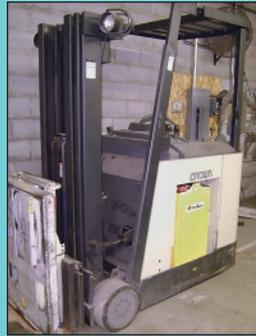
3,700 Lb. Crown Model RC 3020-40 Stand Up Electric Lift Truck
