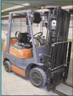
5500 Lb Toyota Model 42 6FGCU25 Solid Tire LP Lift Truck
