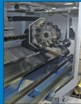
10-Position Tool Turret and Tail Stock
