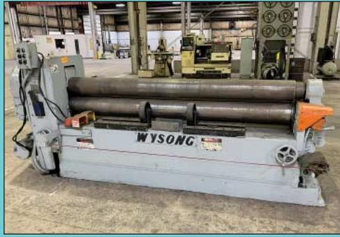
1/4" x 8' Wysong Model F-96 Plate Rolls Hydraulic Plate Bending Rolls
