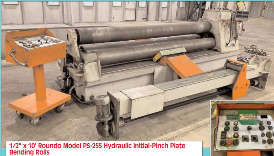
1/2" x 10' Roundo Model PS-255 Hydraulic Initial-Pinch Plate
