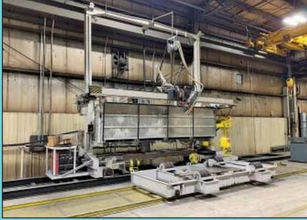
18' Subarc Seam Welding System w/ Lincoln DC-600 Welder, Tank Turning Rolls & 40' Track, 60' Seam Track
