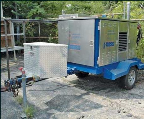
Carolina Equipment Model D44 60-100 "The Aqua Miser" Trailer Mounted Bicarbonate of Soda Stripper
