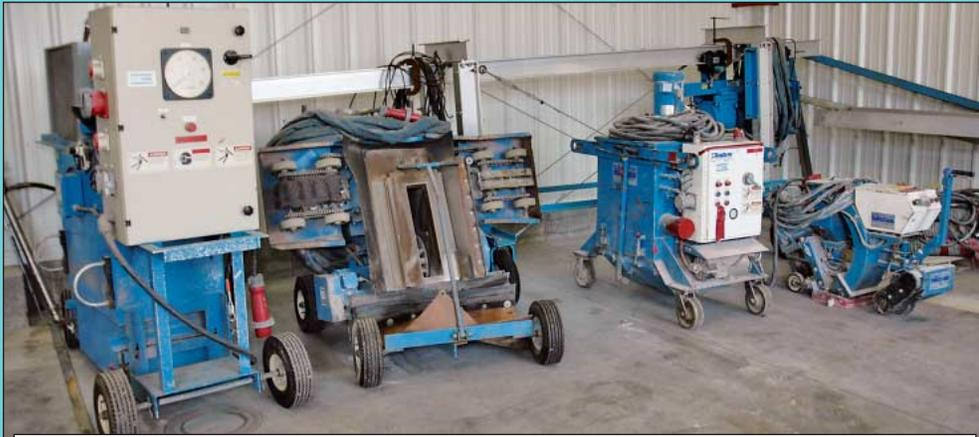
**U.S. Filter Model "Porta Wheel" Vertical Shot Blast Cleaning System**
