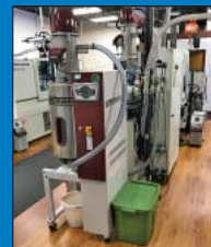
(3) Wittman Dry Max Dehumidifying Dryers
