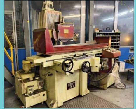
12" X 30" Kent Model SGS1250AHD Hydraulic Surface Grinder
