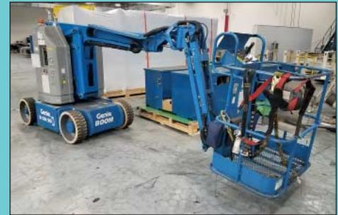
36' Genie Model Z-30/20N Articulated Electric Boom Lift
