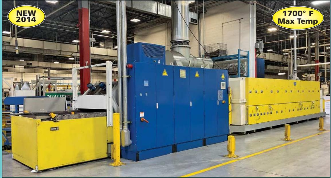
50" Wide Eliino Model FB-125/072/050-08EW.OC Electric Mesh Belt Conveyor Type Heat Treat Furnace
