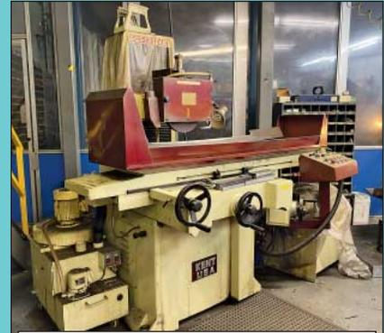
12" X 30" Kent Model SGS1250AHD Hydraulic Surface Grinder
