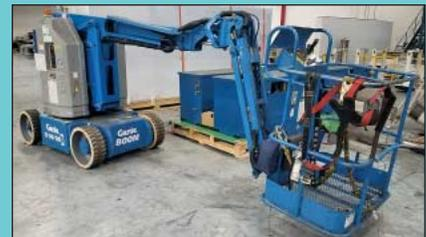
36' Genie Model Z-30/20N Articulated Electric Boom Lift
