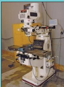
3 HP Jet Model JTM-4VS Variable Speed Vertical Milling Machine
