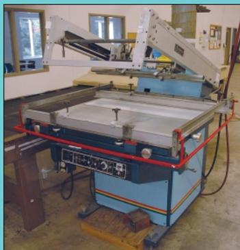
25" X 38" American Screen Printing Equipment Model Tempo 2538 Semi-Automatic Screen Sprinting Machine
