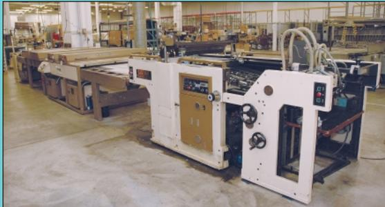
Overall View 28" Sakurai SC-72A Fully Automatic Screen Printing Line w/ Dryer and Stacker
