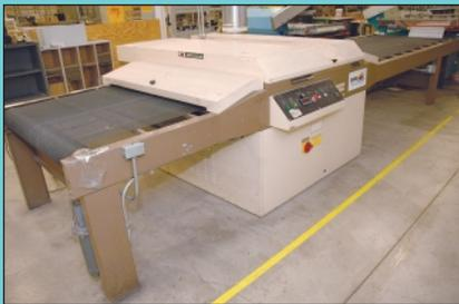
48" Wide SPE Model 3PI-481EC Belt Type Drying Oven
