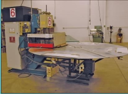
(2) 15KW Thermatron Model F15-25 Pneumatic Press Rotary Table Type RF Sealing Machines
