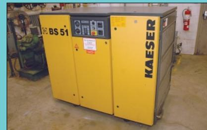
40 HP Kaeser Model BS-51 Rotary Screw Cabinet Enclosed Air Compressor
