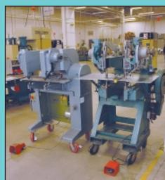
Partial View (2 of 10) Late Model Dual Head Riveters
