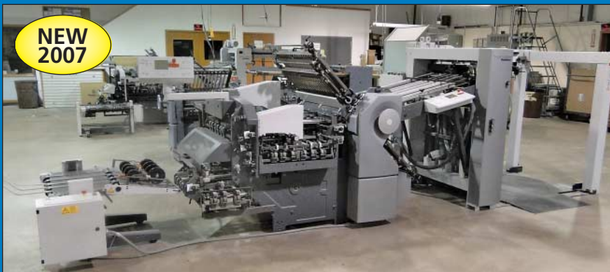
30" X 50" Heidelberg Stahl Model BCUH-78 Knife Folder
