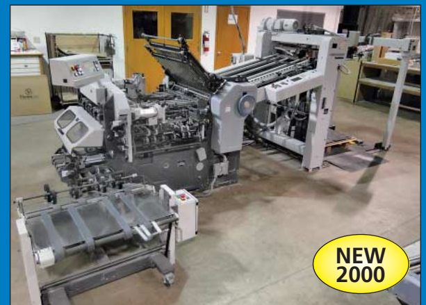
30" X 52" Heidelberg Stahl KD-78 Model KD.2-82/4-KLLPPT Knife Folder
