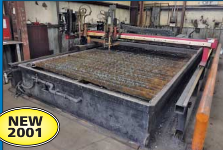
8' x 24' Koike Model PLP 2500 CNC Plasma Table
