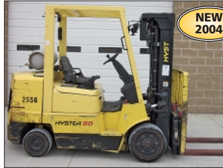
8,000 LB Hyster Model S80XM LP Gas Solid Tire Lift Truck
