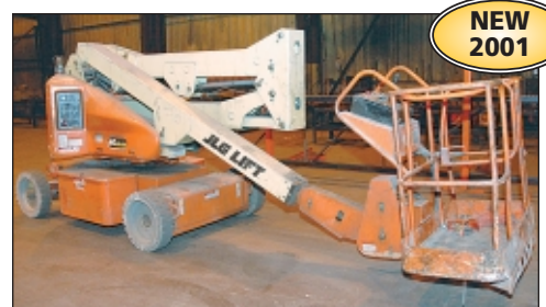
500 LB JLG Model N40 Electric Snorkel Lift
