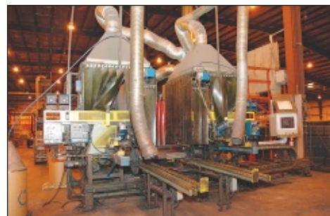
(2) 12' Rumble Automation Automatic Beam End Cap Welding Systems
