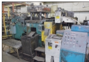
60 Ton Henry & Wright 4-Post Notching Press
