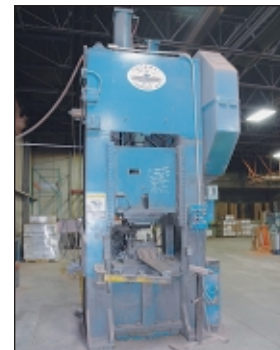
200 Ton Federal Model S1-200-36-42 Straight Side Single Crank Press
