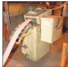
Cooper Weymouth Uncoiler and Straightener
