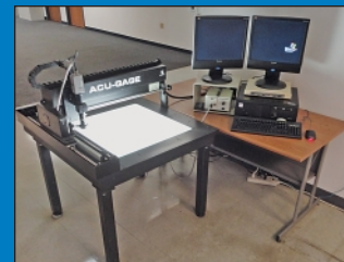
24" Acu-Gage Systems Model AG24-2-LM4 Optical Measuring Machine
