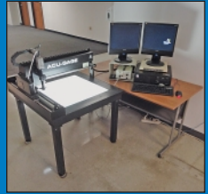
24" Acu-Gage Systems Model AG24-2-LM4 Optical Measuring Machine
