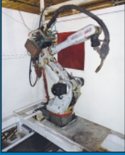
Close Up View Motoman Robot In Welding Cell
