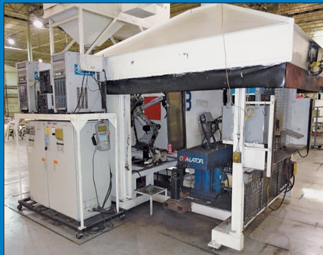
Motoman Two-robot CNC Robotic Welding System
