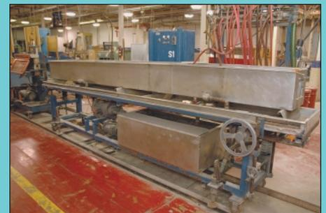
(2) Extrusion Services Inc. Model Vac-Tank Calibration Tables w/ S.S. Tanks
