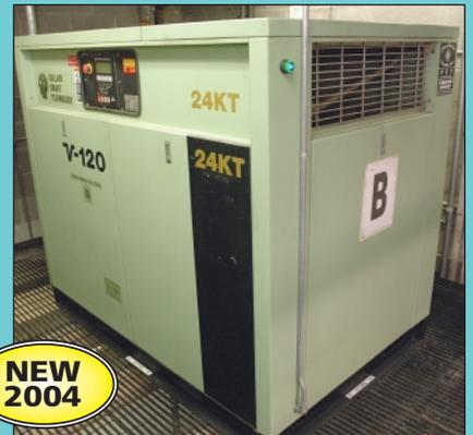
50 HP Sullair Model LS-120-50 HA Rotary Screw Cabinet Enclosed Air Compressor
