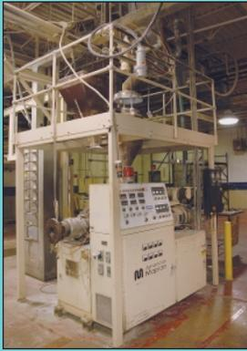
2" American Maplan Model CON-40 Twin Screw Extrusion Machine
