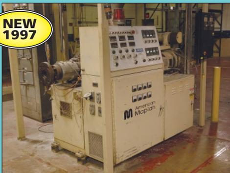
2" American Maplan Model CON-40 Twin Screw Extrusion Machine
